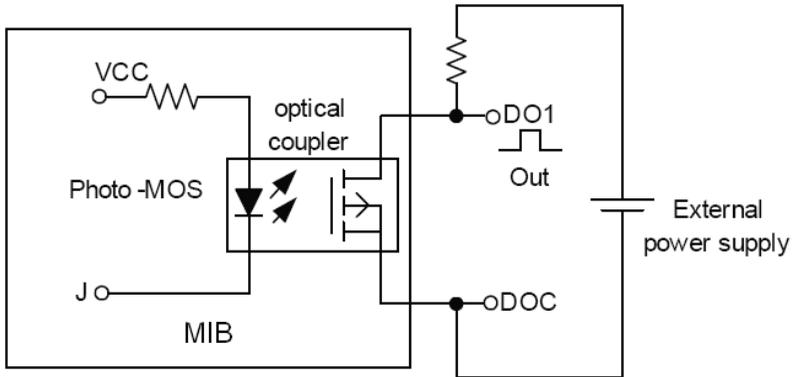
The Max output voltage and current are 250Vac/300Vdc and 50mA. When the digital output is used as over/under limit alarm output High/low limit and alarm time can be set in System parameter settings.
