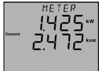
**Note:** when the voltage wiring of the meter is set to 2LL or 3LL, there is no phase power, phase reactive power and phase power factor shown in display.
